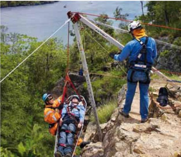
Sideways A-frame Using Pulley Head
