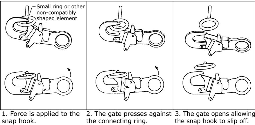
**2.2 COMPATIBILITY OF CONNECTORS:** Connectors are considered to be compatible with connecting elements when they have been designed to work together in such a way that their sizes and shapes do not cause their gate mechanisms to inadvertently open regardless of how they become oriented. Contact DBI/SALA if you have any questions about compatibility.
