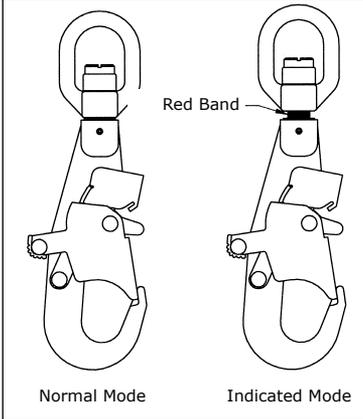
**Figure 12 - Inspection level wind 8102000**
