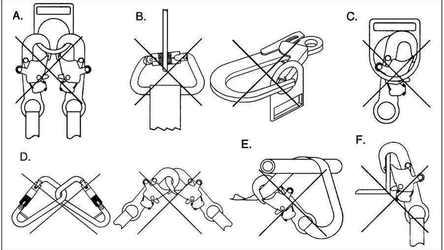
DBI/SALA connectors (snap hooks and carabiners) are designed to be used only as specified in each product's user's instructions. See Figure 4 for inappropriate connections. DBI/SALA snap hooks and carabiners should not be connected:
