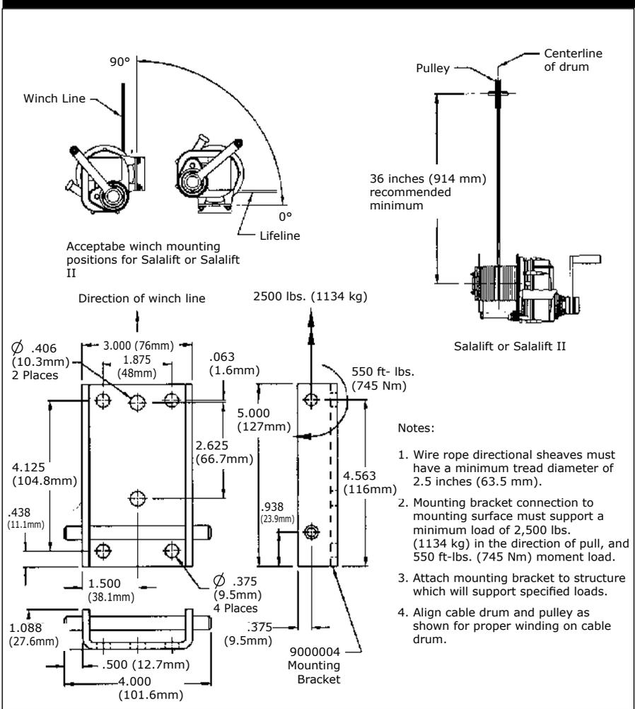
**B. LOAD REQUIREMENTS:** Figure 5 illustrates mounting the winch to the support structure and the load requirements. The mounting bracket must support the loads shown in Figure 5.
