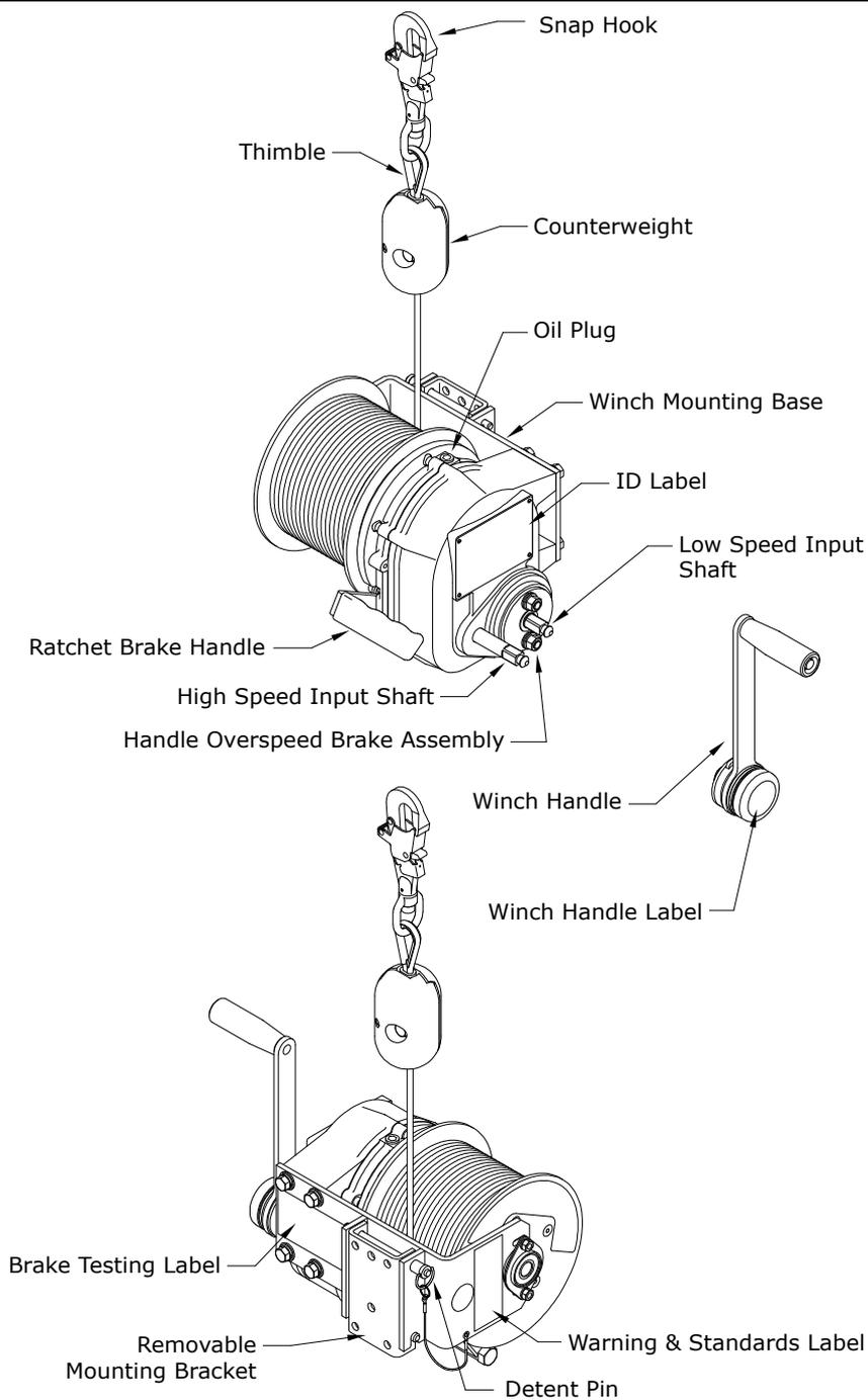
**Figure 2 - 8102001 Series Parts Identification**
