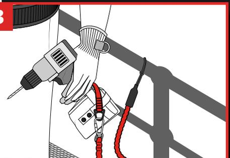
Attach a GRIPPS® tether with an appropriate load rating to the D-Ring on the choke strap.
