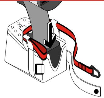
Insert the battery pack (whilst connected to the power tool) into the Battery Catch Holster XL..
