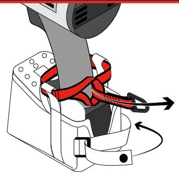
Secure the holster by pulling the strap tightly and clicking the closest button. Ensure the choke strap passes through the three choke guides by passing the D-Ring end through the loop end of the choke.
