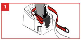
Insert the battery pack (whilst connected to the power tool) into the Battery Catch Holster XL. Insert the battery pack (whilst connected to the power tool) into the Battery Catch Holster XL.
