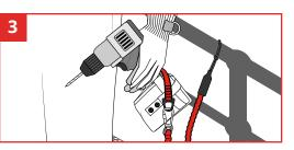
Attach a GRIPPS® tether with an appropriate load rating to the *D*-Ring on the choke strap.
