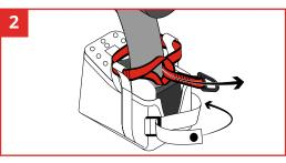
Secure the holster by pulling the strap tightly and clicking the closest button. Ensure the choke strap passes through the three choke guides by passing the D-Ring end through the loop end of the choke.
