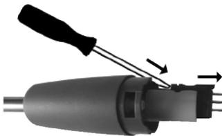
1 Release the probe catch by pressing the key on the probe handle and remove the probe module.
