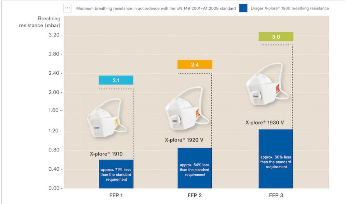
\* All values for inhalation at 95 l/min. The values depicted are average values for the Dräger X-plore® 1900 version in size M/L, based on Dräger's internal testing, measured according to the requirements of the EN 149:2001+A1:2009 standard.
